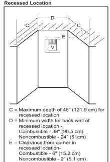
Figure 7 - Minimum Clearances for Termination Cap
